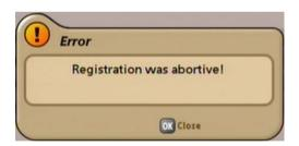
Check your settings (frequency and transmission channel) and if necessary call for expert help.
